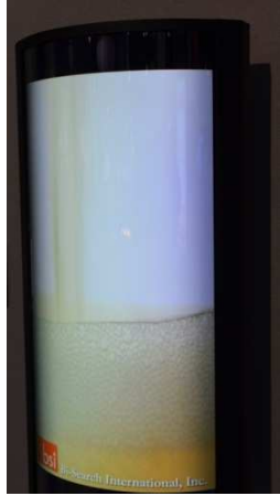
Figure 2. BSI display with LCD resized and curved by TED licensee Tovis of Incheon, Korea. (Photo: Ken Werner)
