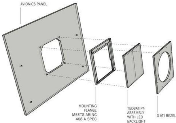
2. Technique for mounting TED3ATIP4 display to surface of avionics panel using proprietary TED flange and bezel. (c. 2014 Tannas Electronic Displays)
