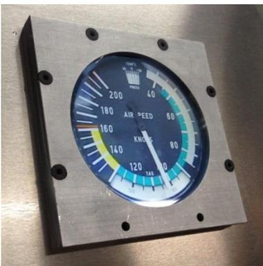
1. TED 3ATI4P display mounted to surface of aluminum panel with proprietary flange. A bezel with a round opening finishes off the round air-speed indicator being simulated by the display. (Photo: TED)
