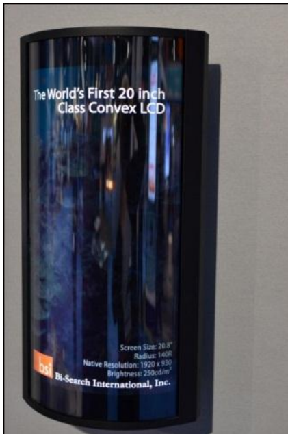
Figure 3. Resized 20-inch glass convex display with 1920x930 pixels. Display by BSI. Panel by TED licensee Tovis Co., Ltd of Incheon, Korea. (Photo: Ken Werner)
