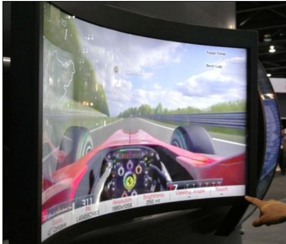
Figure 2. BSI concave display for gaming and simulation applications was resized to 40 inches diagonal and 1880x1056 pixels (Photo: Ken Werner)
